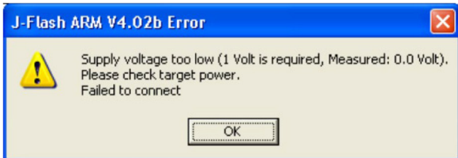
Figure 71: Failed to Connect Error Message
