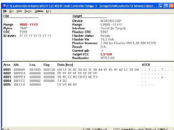
Figure 67: Incorrect Range and Target VCC Fields
